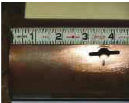
PHOTO 3: The hole for the N connector. Note that the slot either side of the hole is not necessary, although you will need mounting holes for the N connector flange.
