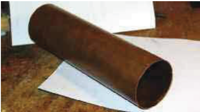
PHOTO 2: Raw 76mm copper tube cut to length.
