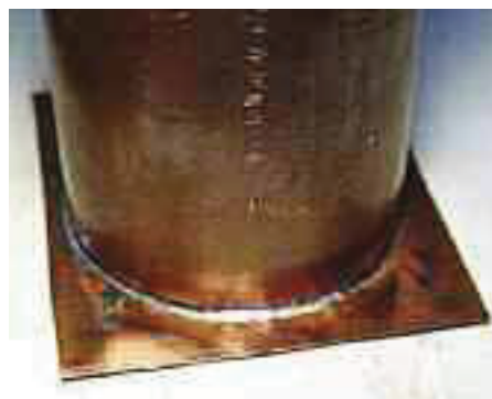
PHOTO 6: The end plate is soldered to the tube. The corners can be trimmed off after soldering.
