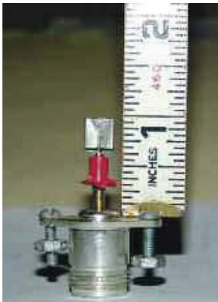
PHOTO 4: The completed feed assembly.
