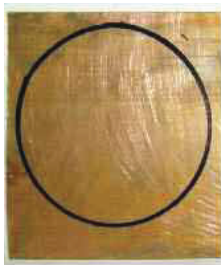
PHOTO 5: The end plate can be any shape as long as it's larger than the outside diameter of the tube.
