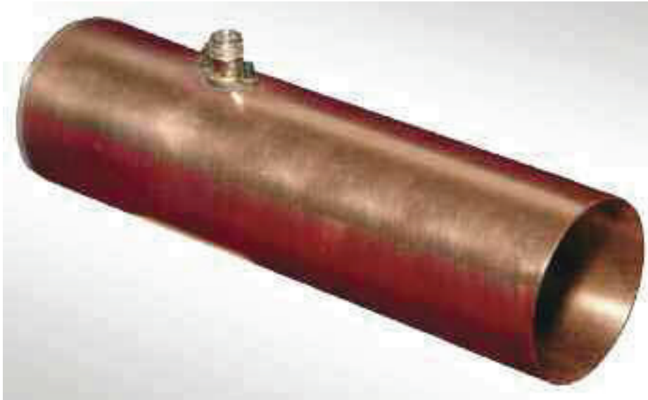
PHOTO 1: The finished basic 2.4GHz tube antenna gives around 9dB of gain.
