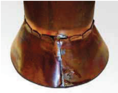
PHOTO 3: Soldering the conical hood to the tube.
